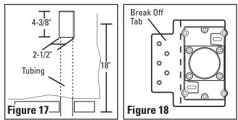
4. Remove the perforated section of the mounting plate (Figure 18) and cement a model CVFE90S short 90° elbow to the mounting plate, facing the correct direction to make the connection to the tubing (Figure 19) (see step 7 in Installing the Tubing section for cementing instructions).
